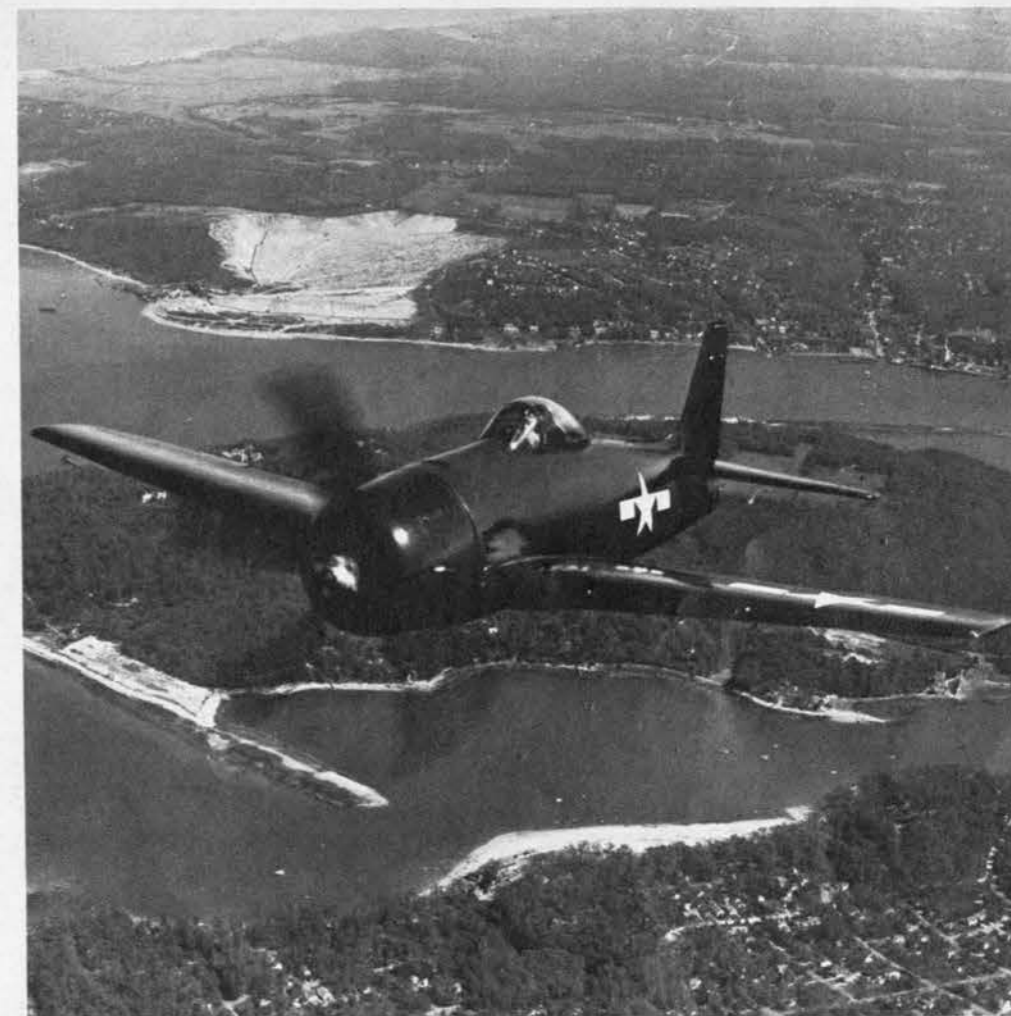
Bearcat combines recognition features from both the Hellcat and Wildcat. Like the F6F it has low mid-wing. Like FM-2, its nose is round, its wing unbroken with dihedral from roots.
